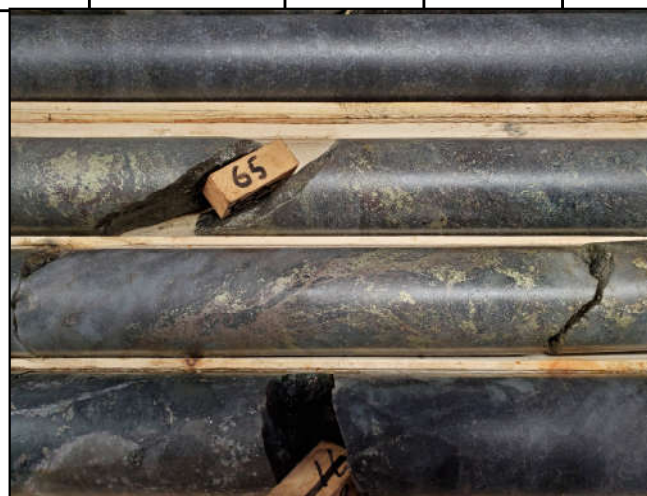
Heavy Chalcopyrite and Sphalerite Mineralization With Subordinate Pyrite From the Conductive Centre
