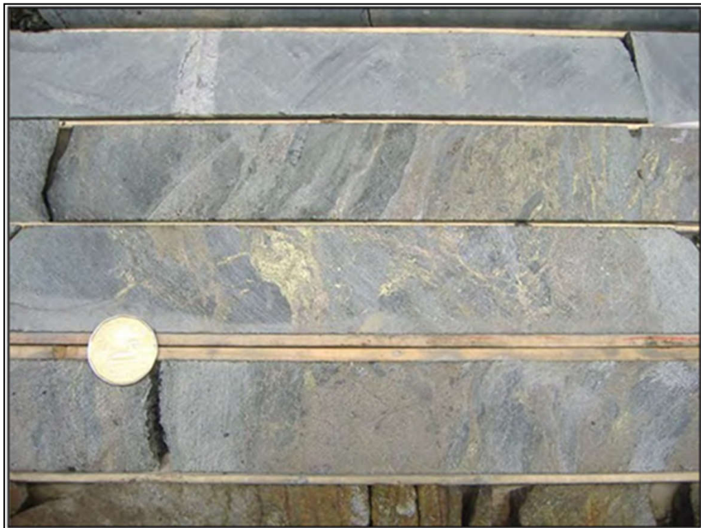
Ultramafic breccia with sulphide matrix of pyrrhotite, pentlandite and chalcopyrite
