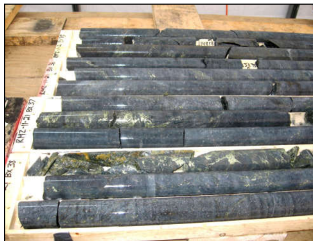
High-Grade Chalcopyrite Mineralization Occurs as Bands, Patches and Heavy Disseminations
