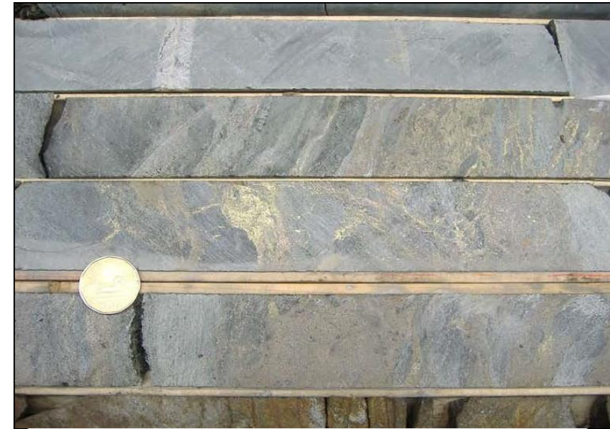
Chalcopyrite, pyrrhotite & pentlandite as nickel sulphide minerals
